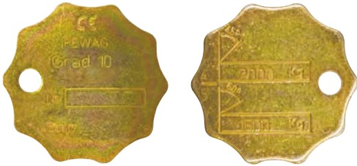
The pewag winner 200 load capacity tag.
