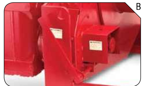
Shown with double compartment and narrow drum width modifications and rotary limit switch.
