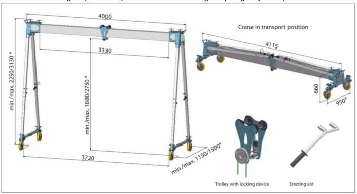
\* Cranes equipped with cross country off-road wheels make the crane 50 mm higher and 100 mm wider.
