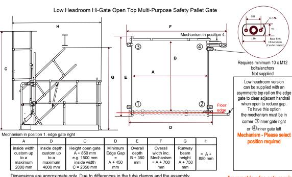
Dimensions are approximate only. Due to differences in the tube clamps and the assembly process, the actual dimensions may vary slightly. Any critical dimensions such as hole fixing centres should be determined when the product is actually on your site. Safe use and installation instructions are provided,
