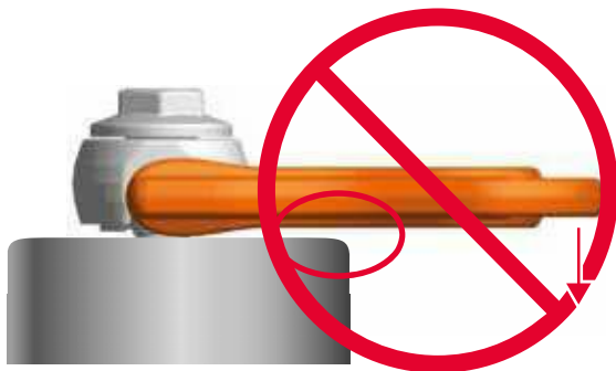
Improper loading as loading ring rests against edges or surfaces
