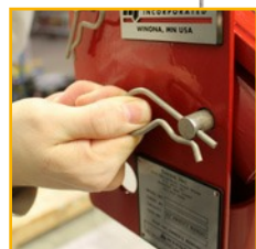
Clevis style pins for quick release, boom adjustments,
