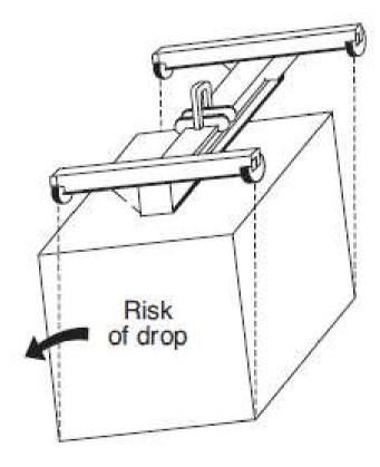
A typical application of this kind might be a container lifted from the base. The lifting beam is connected to the container base by four vertical single leg slings.
