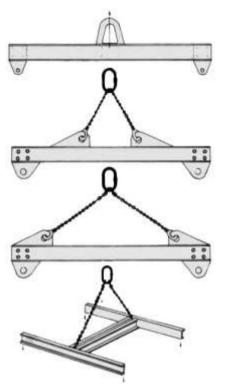
A lifting beam is loaded in bending.
