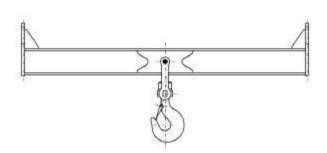
This facilitates tandem lifting. The total lifting capacity can be that of the two cranes less the self-weight of the beam and any allowance for uncertainty in the sharing of the load.
